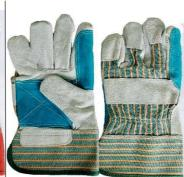
A durable, hardwearing rigger style work glove made from high quality cow side split leather, featuring wing thumb, fully reinforced three fold thumb, fully welted seams, with fingertip protection and knuckle strap. Fully lined for added comfort.
