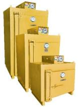
The Drying Oven is used to heat the welding electrodes to a temperature and time specified by the manufacturer to dry a specific type of welding electrode. It reduces the chance for the introduction of hydr-ogen into the weld by removing the moisture from the electrode. The Drying .Oven may also be used as a Keeping Oven as it has a temperature range of 100 - 800 deg. F (38 - 420 deg. C).
